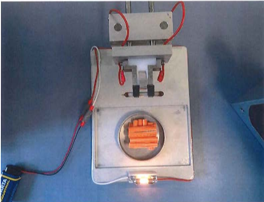
Fig. 13: E-bulb test setup, plan view with connected 9 volt battery
