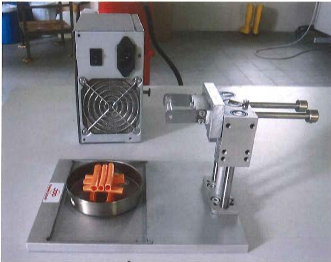
Fig. 11: Test setup side view with stacked cable insulation as combustion material, ampule holder with E-bulb in initial position outside of the fire dish; here: virtually identical test setup from the year 2013
