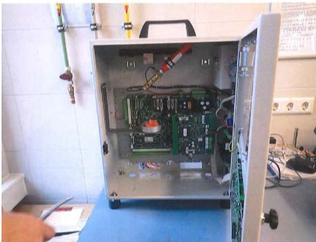
Fig. 7: Interior of the FACU housing with functionally ready S-R-AMFE mini extinguisher and combustion material (cable insulation) for the thermal triggering test (fire dish below the extinguisher)
