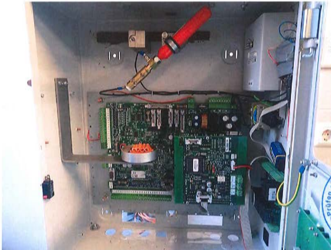
Fig. 18: Test setup for thermal triggering directly before igniting the combustion material
