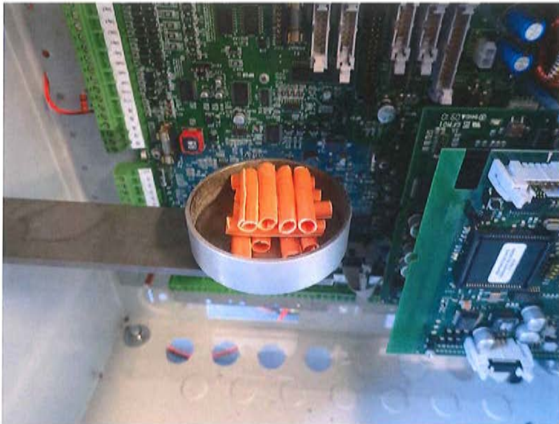
Fig. 19: Introduced fire load = 12 pieces of cable insulation of the type Draka UC900 SS23 Cat.7S/FTP 2x4P LSHF (Low Smoke Halogen Free) at 4 cm in length
