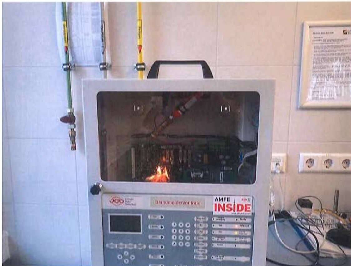
Fig. 23: Mini extinguisher S-R-AMFE has triggered, status indicator switched from "Ready" to "Triggered"
