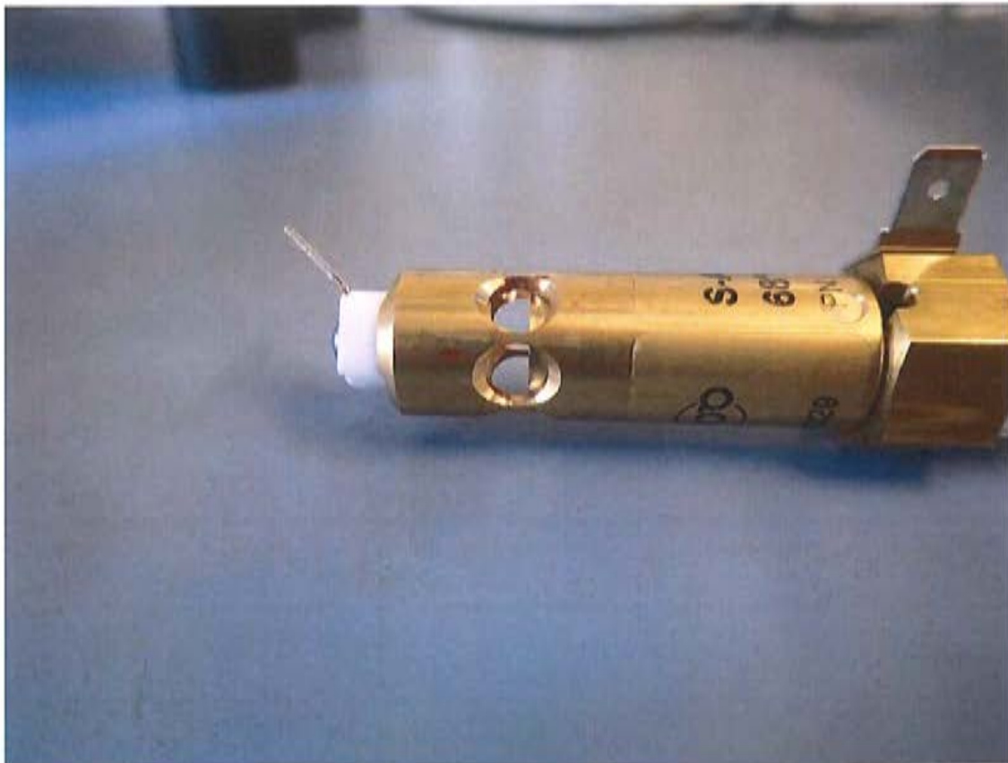
Fig. 25: S-R-AMFE control and triggering unit after triggering, thermo bulb has burst
