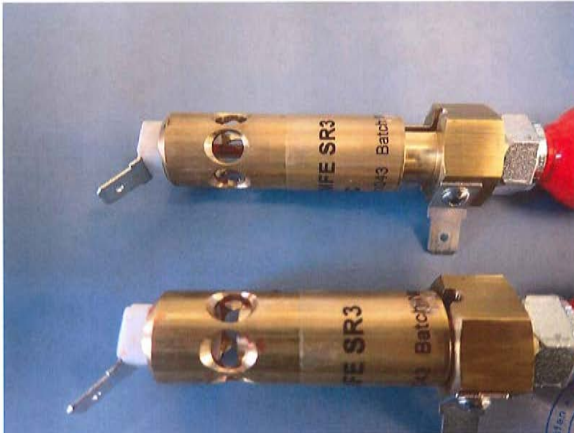
Fig. 26: S-R-AMFE control and triggering unit prior to and after triggering
